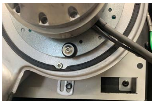
Fig. 15: Installing the ADM
