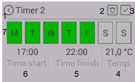
Fig. 46: Creating heating times
