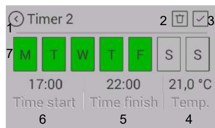
Fig. 31: Creating heating times
