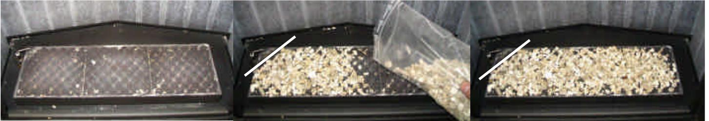
Ensure that you do not scatter vermiculite past the white line in relation to the ionisation rod in connection with the ignition.
